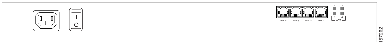
Figure 2-3 Cisco Unified Videoconferencing 3522 BRI Gateway: Rear Panel
